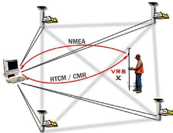
Figure 3 *The VRS measurement process*
